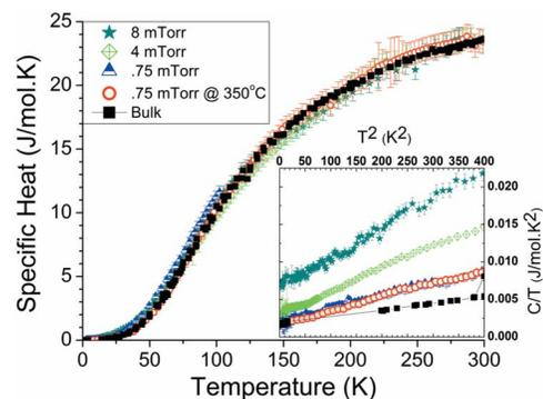
FIG. 1. (Color online) Specific heats of different sputtered Cr films compared to bulk data. Inset shows the  $C/T$  vs  $T^2$  plot used to obtain the Debye temperature and Sommerfeld coefficient.
