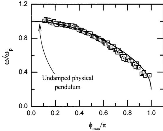
FIG. 3. A plot of the oscillator frequency (Ref. 16) as a function of phase angle. An ideal rigid pendulum (without damping) would follow the smooth curve drawn as a solid line (Ref. 13). The data are the average of approximately 50 transient ring downs.
