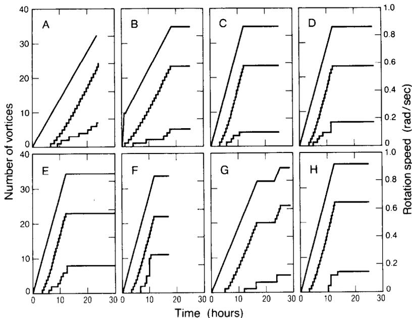
Fig. 10. The results of eight slow acceleration trials. For each trial the upper curve gives the rotation speed (right scale), the middle curve gives the predicted equilibrium number of vortices (left scale) and the lower curve gives the observed vortex number (left scale). All are plotted vs. time.
