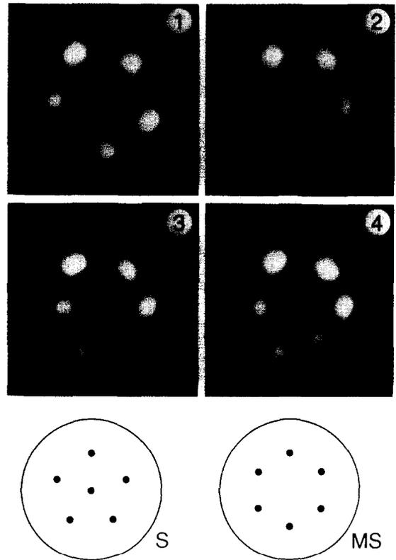
Fig. 5. Photographs 1 through 4 are sequential multiple exposure prints. There are 30 frame exposure and each corresponds to 6.7 min of filming at 0.47 rad/s. Below these are shown the predicted S and MS configurations for a rectilinear array of six vortices as given in ref. 8.
