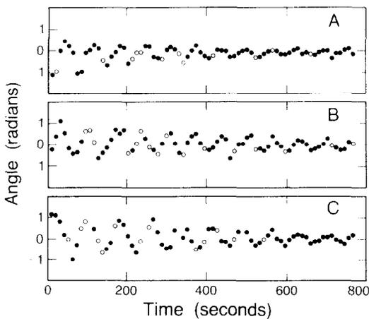
Fig. 8. The angular orientation of two-line arrays plotted vs. time for three different spin-ups, all to a rotation speed of 0.364 rad/s. The open circles are points which have been determined on the basis of a single vortex image, as discussed in the text.
