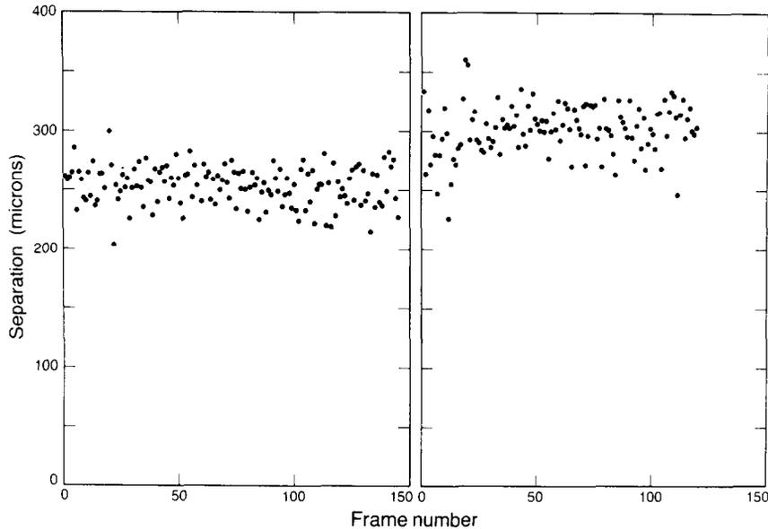
Fig. 6. The separation of the vortices in a two-line array plotted vs. film frame number for two successive spin-up trials. The rotation speed was 0.364 rad/s for both. The time between film frames was 10.6 s.
