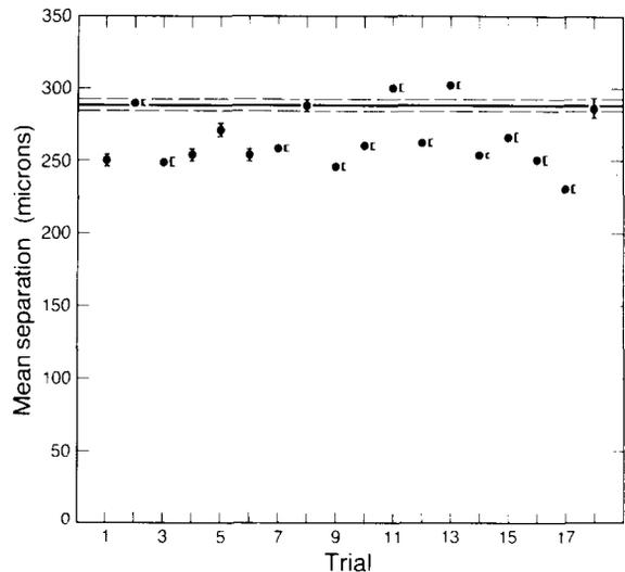
Fig. 7. The time averaged separations of the vortices in two-line arrays produced by independent spin-ups to a rotation speed of 0.364 rad/s. The data are plotted vs. the spin up trial number (chronologically ordered). The solid line is the predicted separation for rectilinear vortices and the dashed lines indicate the uncertainty in this prediction, as explained in the text.
