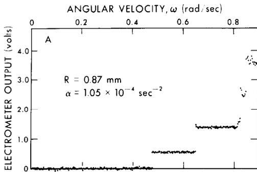
Fig. 1. A plot of charge trapped on vortices vs. angular velocity of the rotating vessel. The step-wise transitions signal the appearance of an additional vortex line.
