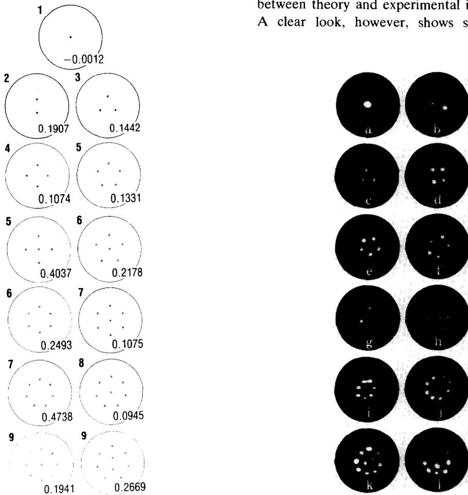
Fig. 4. On the left are displayed the predicted stable and metastable arrays of quantized vortices. The number below each array is a dimensional free energy characteristic of that pattern. On the right are displayed the stationary patterns observed in the experiments.
