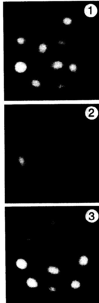
Fig. 3. A sequence of multiple exposure prints. Each print corresponds to 10.6 min of filming (60 frames) at a rotation speed of 0.59 rad/s. Note the slight changes in the array configuration between photographs 1 and 3.
