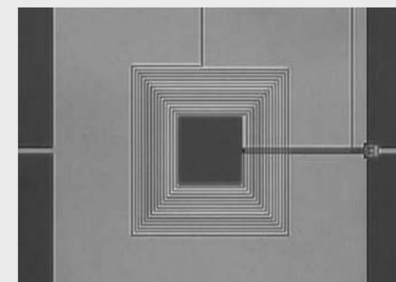
Today's SQUIDs are fabricated using a wafer scale process and photolithography.
