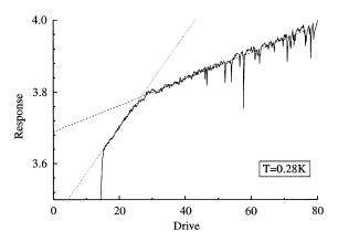
Fig. 1. The two distinct slopes in the supercritical regime indicate that trapped circulation among the apertures is slowly unwound as the drive is increased. The units are arbitrary, but consistent with Fig. 2.
