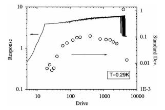
Fig. 2. This response curve shows the progressive increase in the number of phase slips (per half-cycle) as the drive is ramped up. The sudden onset of collapse events occurs at  $\sim 1000$  times the critical drive.
