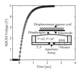
**FIGURE 1.** Displacement sensor voltage output versus time and a schematic of the experimental cell. The heater is turned on at time t = 0 sec. The temperature across the aperture array relaxes to a steady state value  $\Delta T_f$ , determined mainly by thermal conduction through the inner cell walls. The diaphragm relaxes to a new position corresponding to the fountain pressure  $\Delta P_f = \rho s \Delta T_f$ .
