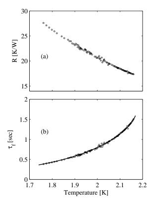
**FIGURE 2.** (a) Thermal resistance *R* from the measured fountain pressure  $\Delta P_f$  versus temperature. *R* is likely determined mainly by conduction through the thin, large area diaphragm. Heat transport by normal flow through the apertures is taken into account separately, and is small compared to thermal conduction. (b) Fountain transient time constant  $\tau_f$  versus temperature, data (circles), and fit (line), from which  $A^2/k$  and *V* are determined.
