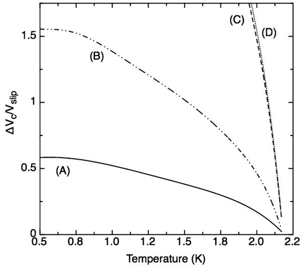
If the apertures used in [15] are treated as circles whose radii give the same areas as the apertures, their effective lengths come out to be 265 nm, 883 nm, and 845 nm. The same analysis gives  $l_{\text{eff}} \sim 75$  nm for the apertures of Hoskinson et al. The effect of having smaller  $l_{\text{eff}}$  (and therefore bigger  $v_{\text{slip}}$ ) is apparent in the result.
