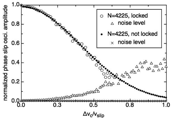
to be the same for all the apertures. For the case of 4225 locked apertures, we simply force all the apertures to slip whenever the critical velocity is reached in some aperture.
