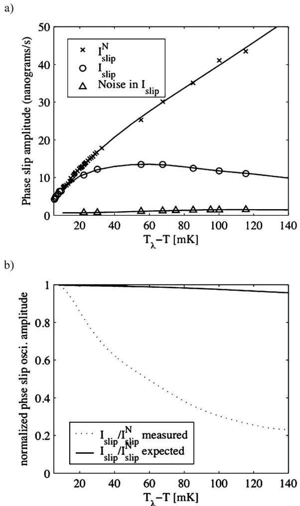
lowered. A dotted line in Fig. 5b is  $I_{\text{slip}}/I_{\text{slip}}^N$ , which is an observed oscillation amplitude normalized so that the expected value  $I_{\text{slip}}^N$  is taken to be 1. (Fitted curves to the data in Fig. 5a were used to produce this plot.) A solid line in Fig. 5b is the simulated  $I_{\text{slip}}/I_{\text{slip}}^N$  with thermal fluctuation in  $v_c$ .
