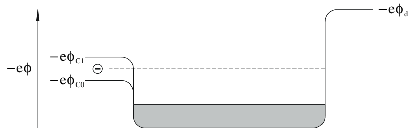
Figure 3.4: Radial position trapping model.
