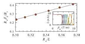
FIG. 2 (color online). (Inset) The beam current collected on successive trap elements, beginning (at  $\beta_q = 0$ ) with the Faraday Plate and ending (at  $\beta_q > 9$  T/m) with cylinder 1, as a function of the quadrupole field  $\beta_q$ . (Main panel) The normalized quadrupole field that maximizes the current on cylinders 1–6, as a function of the distance of the cylinders from the filament front. All measurements are at  $B_s = 0.2$  T.
