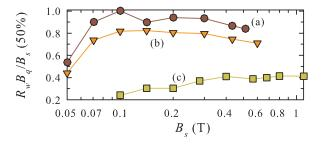
FIG. 5 (color online). The quadrupole field strength at which half the initial ( $\beta_q = 0$ ) charge is lost as a function of the solenoidal field, for a 1 cm grounded trap length that is (a) not briefly lengthened, (b) briefly (2 ms) lengthened to 4.08 cm, and (c) briefly (2 ms) lengthened to 7.08 cm. Once the solenoidal field is greater than about 0.1 T, the loss is roughly independent of the solenoidal field.
