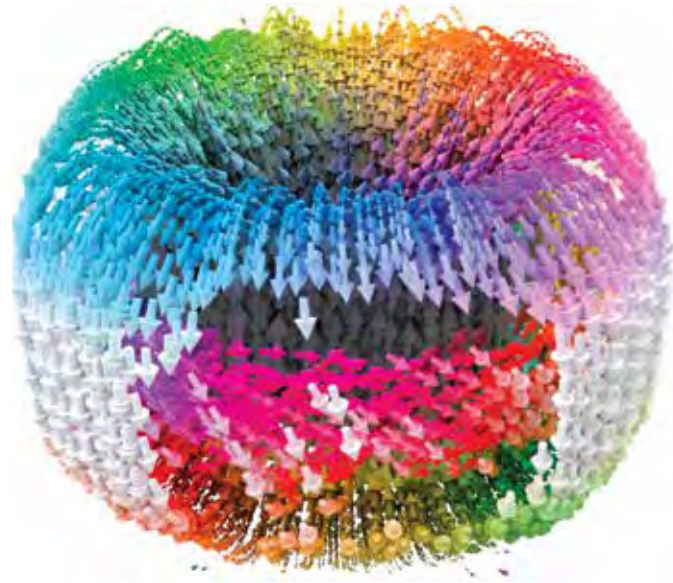
Simulation of a single polar skyrmion. Red arrows signify left-handedness. Other arrows represent the angular distribution of the dipoles. CREDIT: RAMESH TEAM
